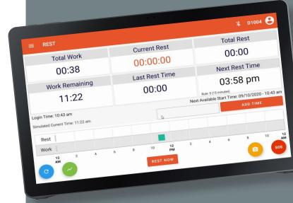
The Driver's on-board tablet requires the driver to log on to the system to do both vehicle and driver health checks. It then monitors the drivers adherence to work and rest times required by the National Heavy Vehicle Regulator.
